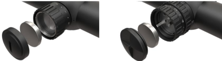
When changing the battery for the MeoStar R2 riflescope, it is necessary to set the illuminator knob to level 8 (maximum). Any other procedure will not guarantee the correct functioning of the illuminator!
